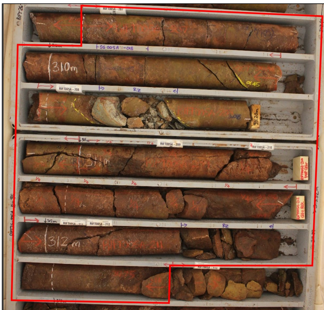
Image 1. RIFT26-005A interval of 3.25 m from 309.5 m to 312.75 m (red box) averaging 4.61% REO, including samples RIFT005A-207 (4.46% REO over 0.98 m), RIFT005A-208 (6.59% REO over 0.52 m), RIFT005A-209 (3.26% REO over 0.96 m) and RIFT005A-211 (5.12% REO over 0.79 m)
