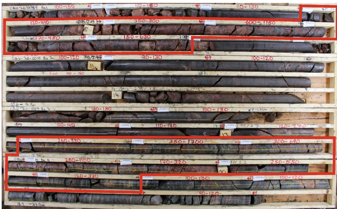
Figure 4. Drill core (NQ 47.6 mm diameter) photos from hole CRV-26-009 highlighting intervals of anomalous radioactivity, alteration, and structure between 7.5 m to 21.0 m depth.
