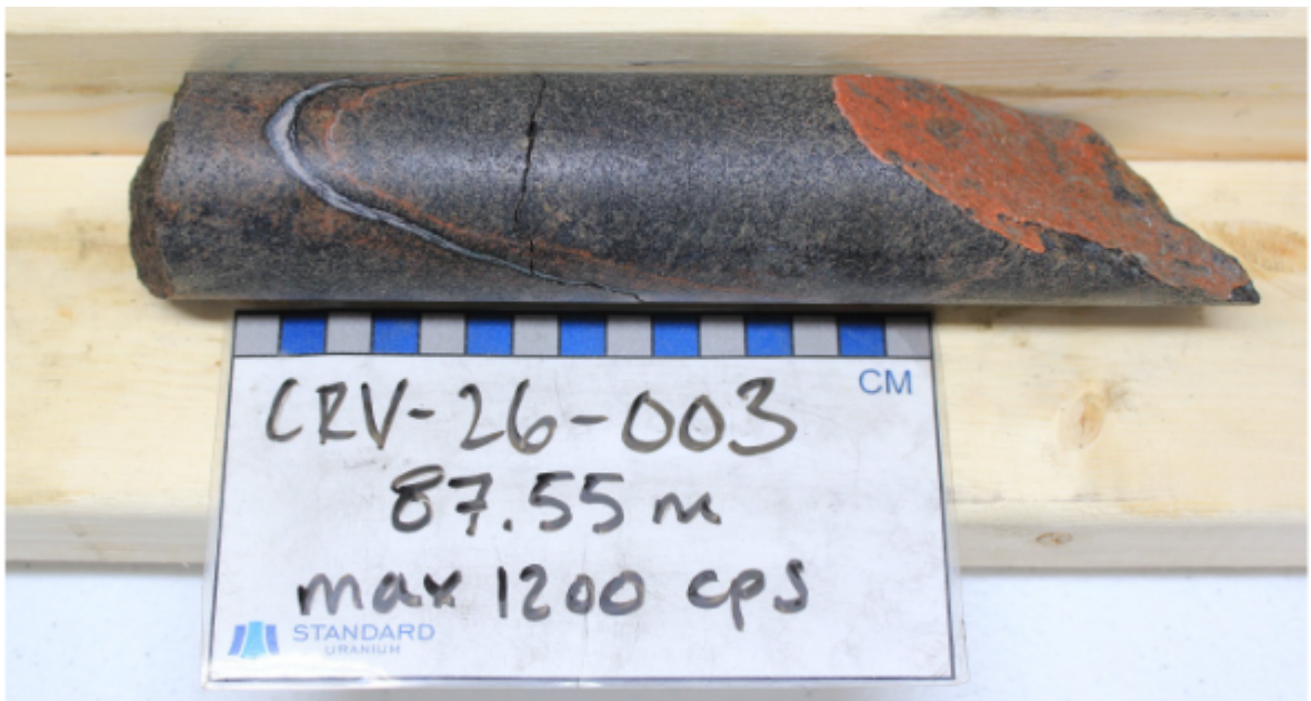
Figure 3. Drill core (NQ 47.6 mm diameter) photo from hole CRV-26-003 highlighting cross-cutting carbonate vein and associated hematite alteration hosting radioactivity up to 1,200 cps at 87.55 m.
