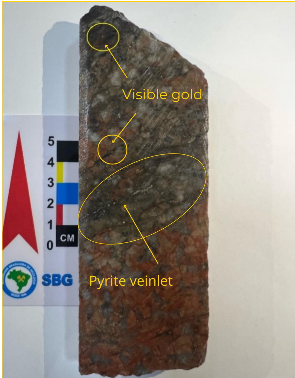
FIGURE 5: HOLE 22ZS014 – VISIBLE GOLD IN MILLIMETRE-SCALE SILICIFIED VEINLETS CROSS-CUTTING HYDROTHERMALLY ALTERED PERTHITIC GRANITE FROM 170.24 TO 171.0 METRES
