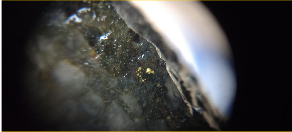
FIGURE 6: HOLE 22ZS011 – VISIBLE GOLD IN CENTIMETRE-SCALE CROSS-CUTTING SILICIFIED VEINLET WITHIN HYDROTHERMALLY ALTERED PERTHITIC GRANITE
