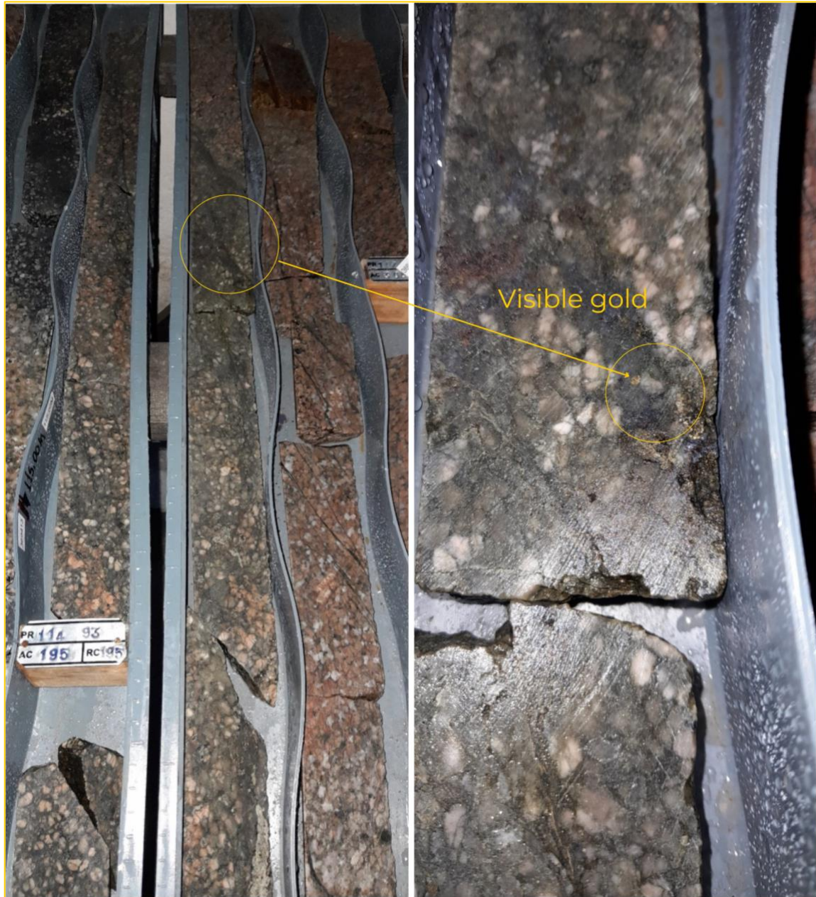
FIGURE 7: HOLE 22ZS011 – VISIBLE GOLD IN CENTIMETRE-SCALE SILICIFIED VEINLETS CROSS-CUTTING HYDROTHERMALLY ALTERED PERTHITIC GRANITE FROM 115 TO 118 METRES (width of core is 4.9 centimetres)
