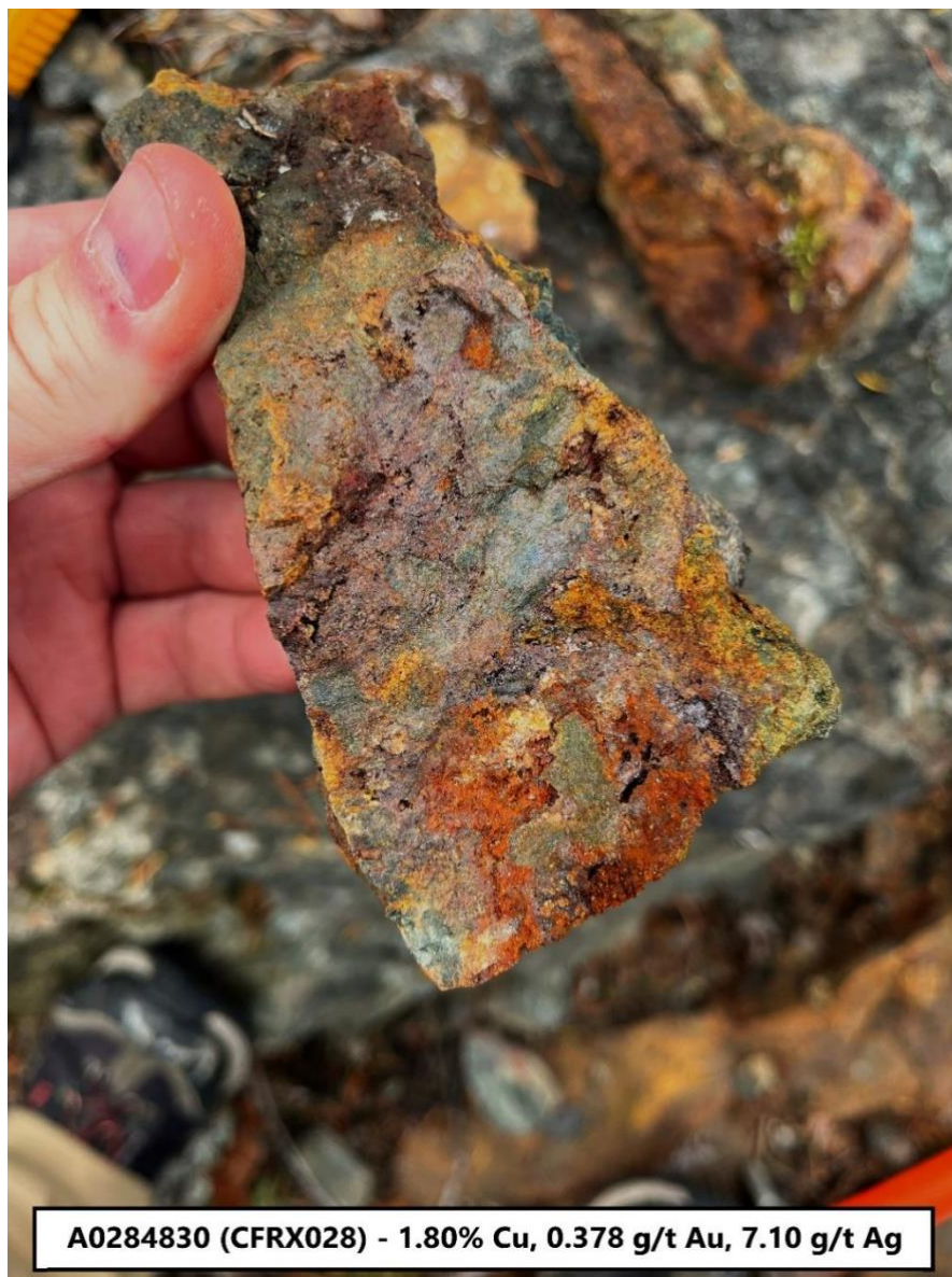
Figure 5: Sample CFRX028, a highly mineralized and altered mafic pillow basalt from the surface exposure of the MGZ. Potentially the feeder zone for the more laterally extensive and more mineralized VMS horizon at depth.
