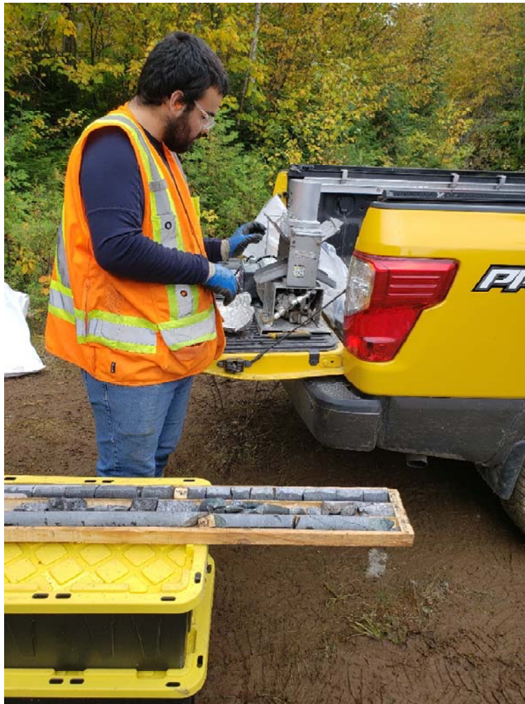
Figure 13 – GMG’s technician uses the hydraulic core splitter to split the core into two halves.
