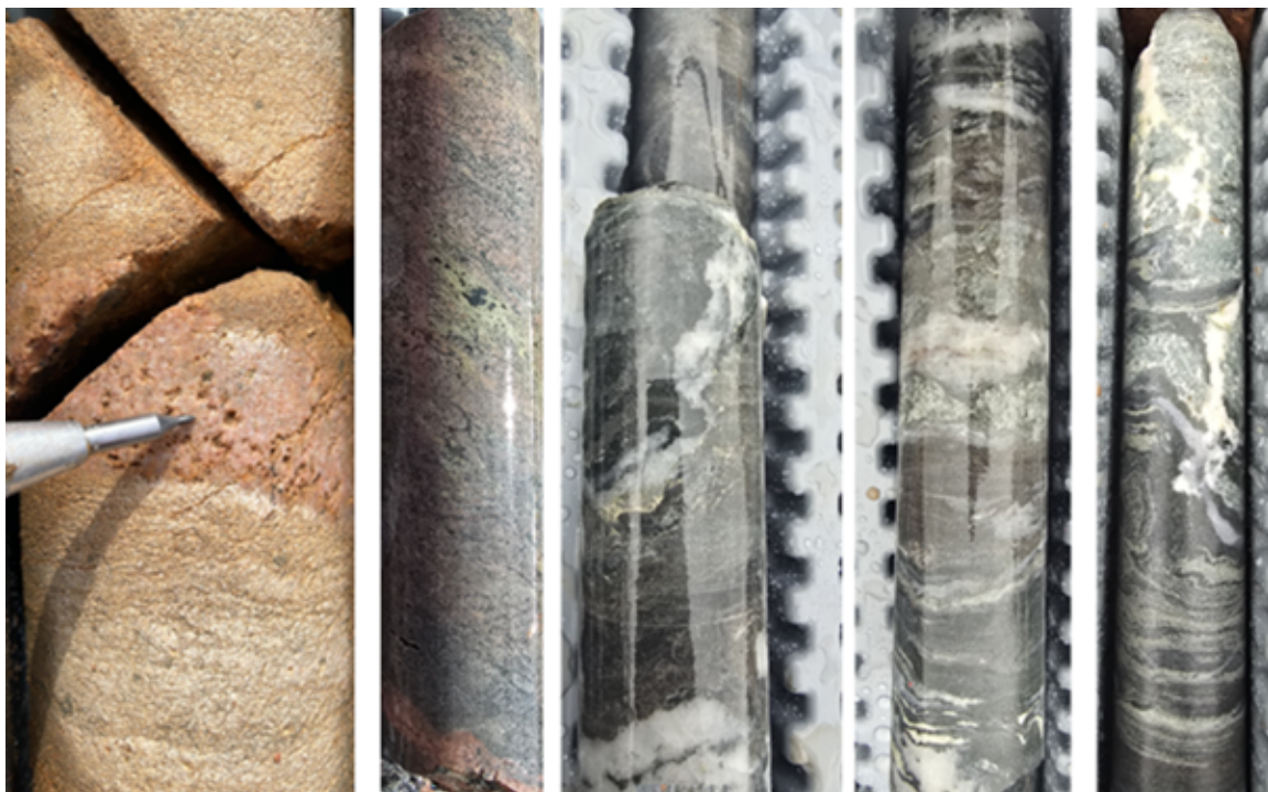
Figure 3. From left to right: 25DDH-SEL-018 at 71m, relic boxwork pyrite in quartz vein in oxidized zone. 25DDH-SEL-018 at
