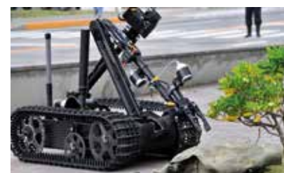
A Mk. II TALON robot from Japan-based Explosive Ordnance Disposal Mobile Unit 5, is used to inspect a suspicious package during a force protection and anti-terrorism training exercise at a United States Navy base in Japan. The exercise trained first responders and support personnel how to react to an improvised explosive device scenario.
