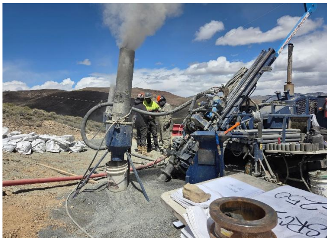
Reverse Circulation drill rig at the Wildhorse Project’s Rattlesnake Zone in Mineral County, Nevada
