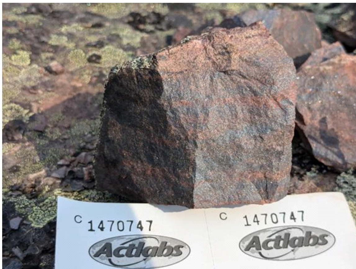
Figure 3: Sample 1470747: Strongly magnetic blue-grey and red banded chert with pervasive sparkly specular hematite
