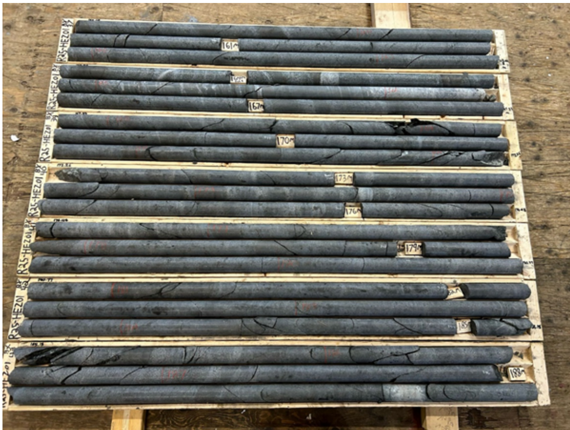
Figure 5: Layering sequence of magnetite ranging from 2-10 inches per band over an almost 30m run of drill hole R25-HEZ-01
