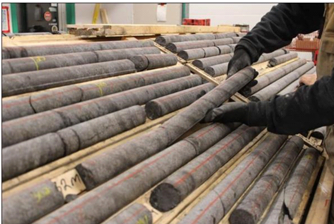
Figure 2: Image of drill core from hole R-0014 highlighting the consistent and extensive rhythmic oxide layering.
