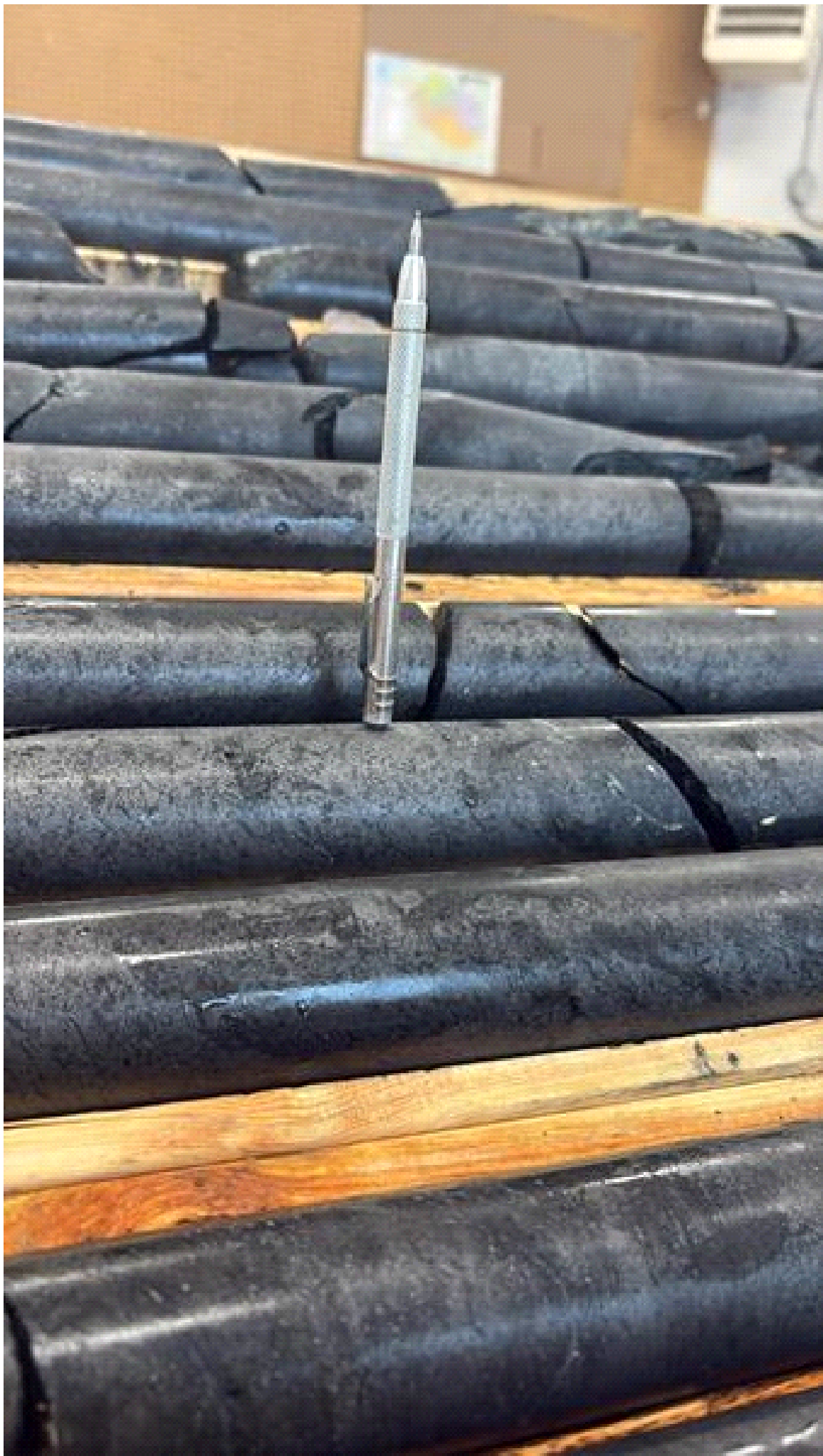
Figure 3: Drill core from hole R-0016 with magnet pen standing straight up highlighting the high degree of magnetism from the oxide rich core.
