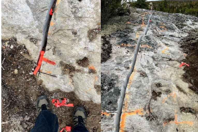
Figure 53: Channel sampling at pegmatite discovery where chip samples were taken by GoldMinds.
