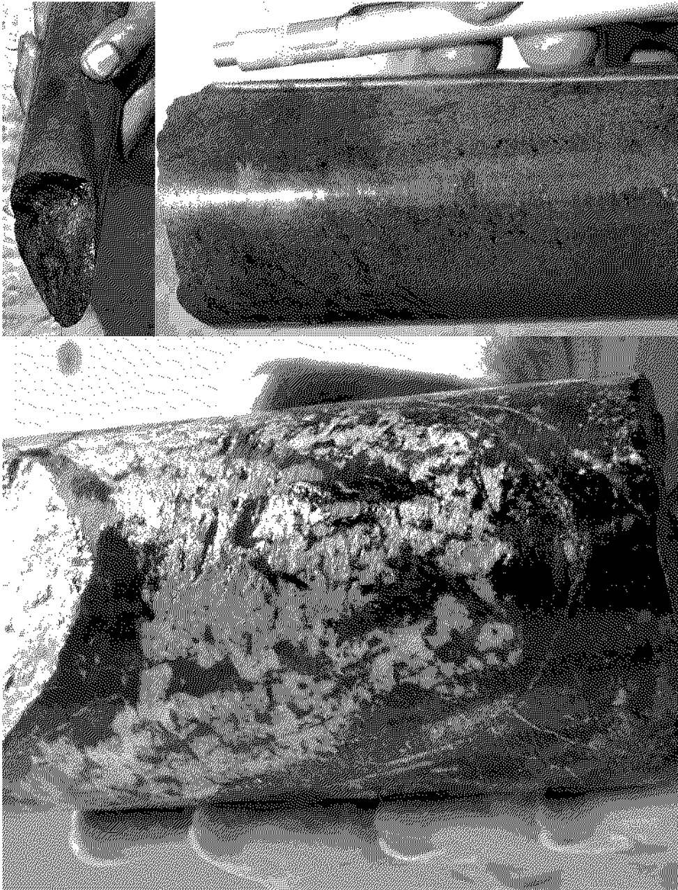
Figure 1. Examples of copper sulphide mineralisation in the Woodchuck drillhole (blue = bornite, yellow = chalcopyrite)
