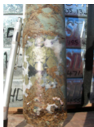
Sphalerite, chalcopyrite and pyrite mineralisation in PDDD2 (sample from 992.5m)
