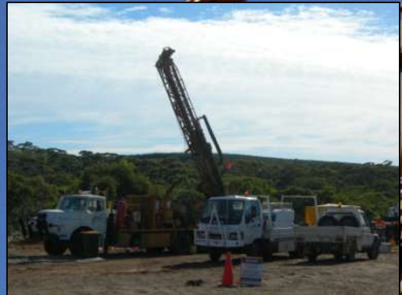
Diamond drill rig at Kohinoor Gold Mine
