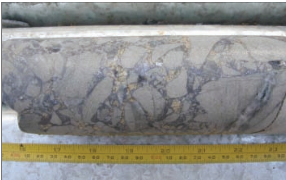
Galena (silver-grey) and sphalerite (light brown) matrix breccia in greywacke
