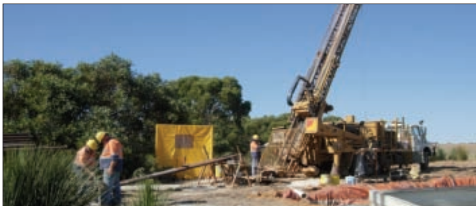
Diamond drill rig at Bonaventura prospect
