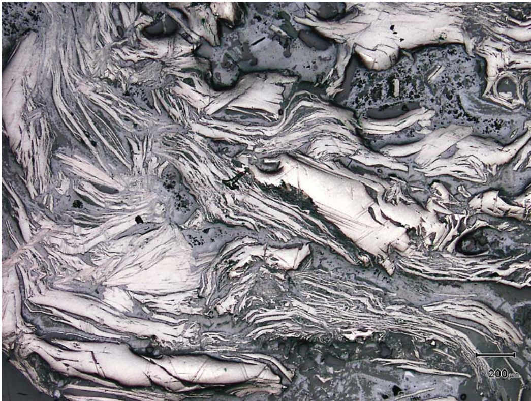
Plate 5. Hole WG031 66-67m. General view of coarse flake graphite. (Note scale bar 200 micron = 0.2mm).
