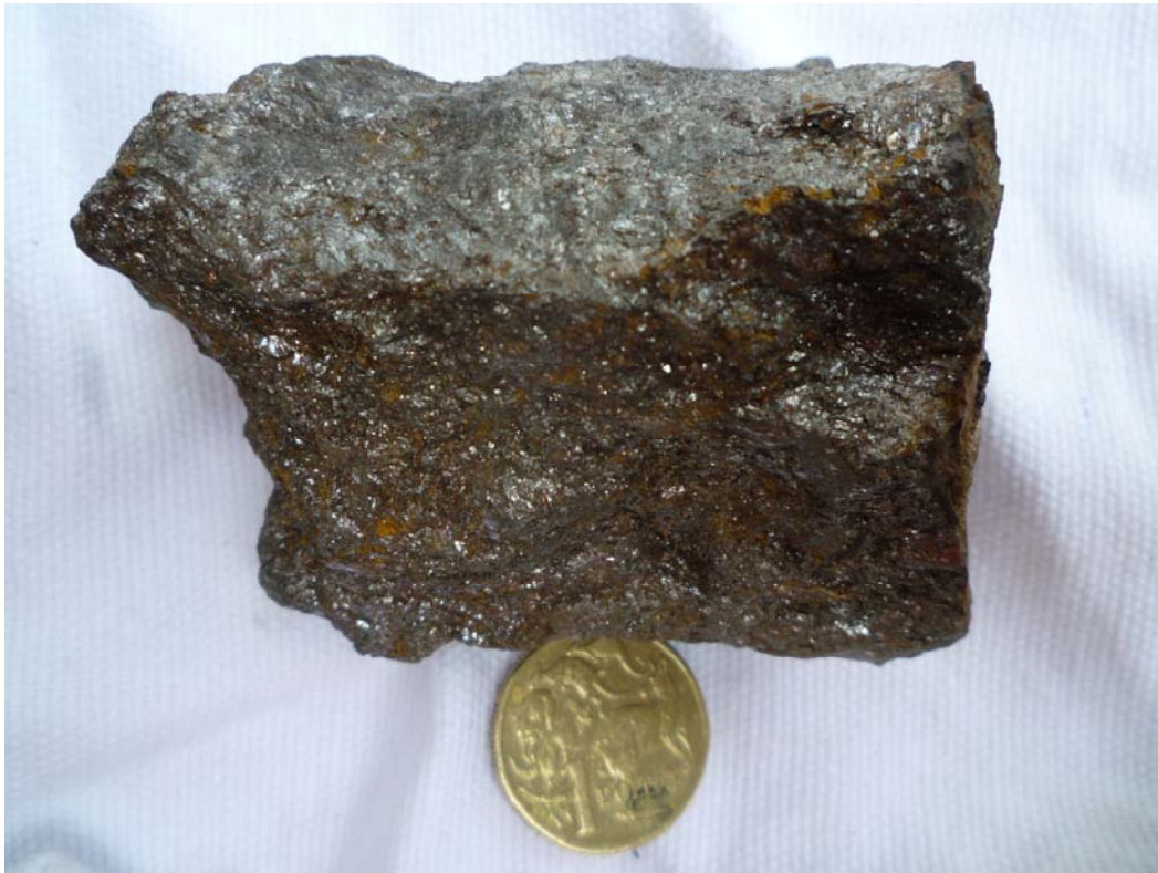
Plate 1. Graphite rich gneiss from Wilclo South. Shiny minerals are coarse flake graphite.
