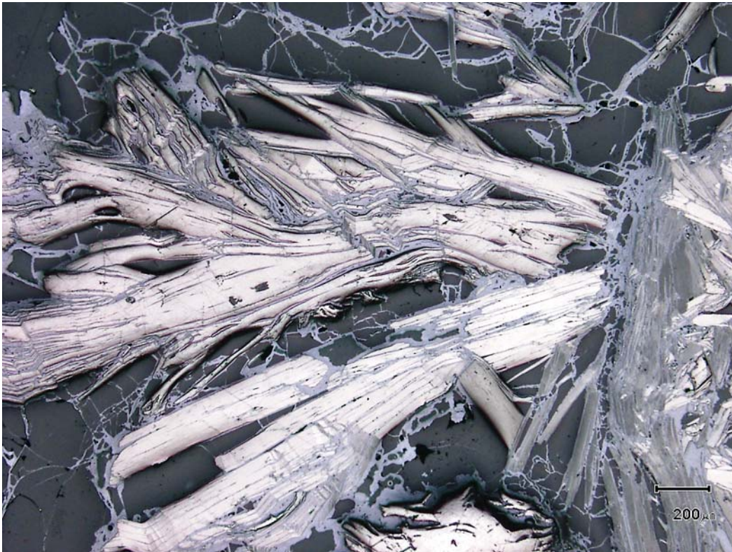
Plate 3. Detailed view of coarse flake graphite from surface sample from Wilclo South. (Note scale bar 200 micron = 0.2mm).
