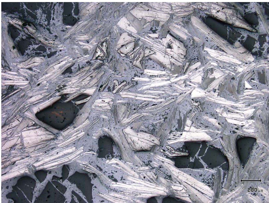
Plate 2. Coarse flake graphite from surface sample from Wilclo South. (Note scale bar 200 micron = 0.2mm). Graphite is intergrown with quartz, limonite and carbonate.
