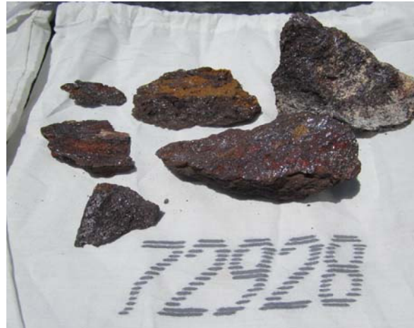
Plate 2. Sample of visible coarse graphite from an outcrop at Wilclo South
