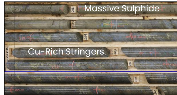
Zone where the massive sulphide transitions into the stringers with no gaps
