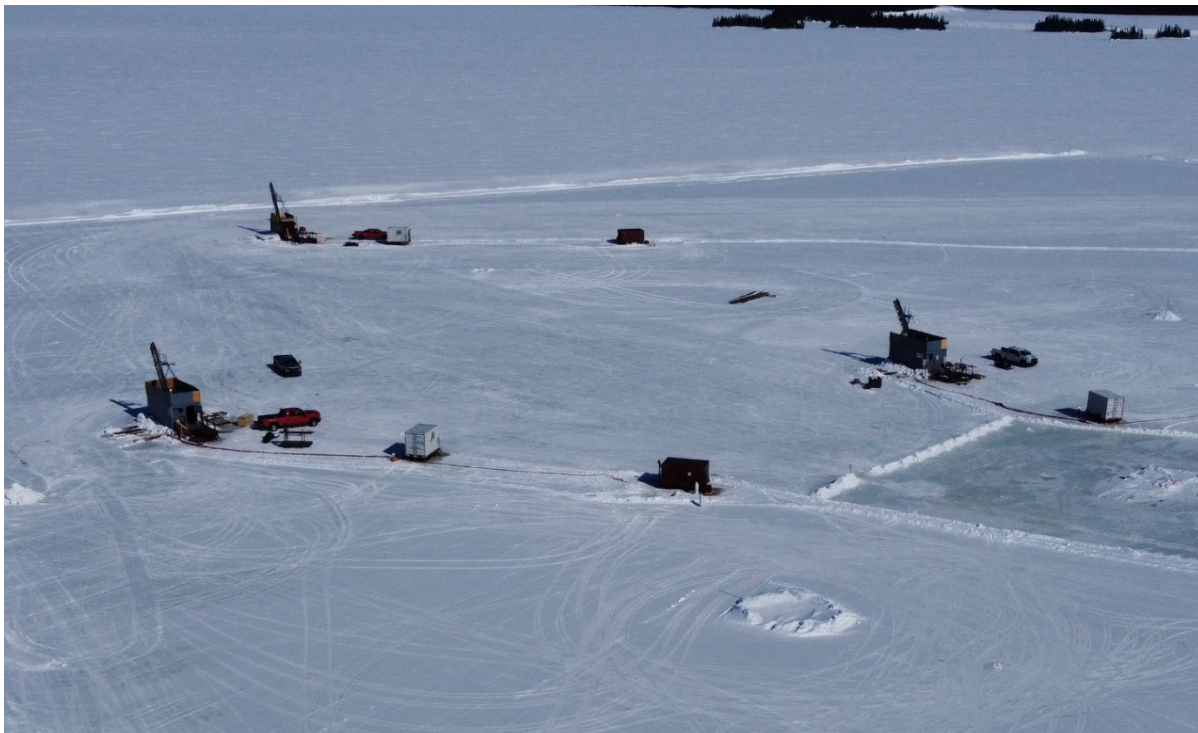
Figure 2: Three drill rigs completing the Golden Eye resource conversion program on the engineered ice pad (March 2026).
