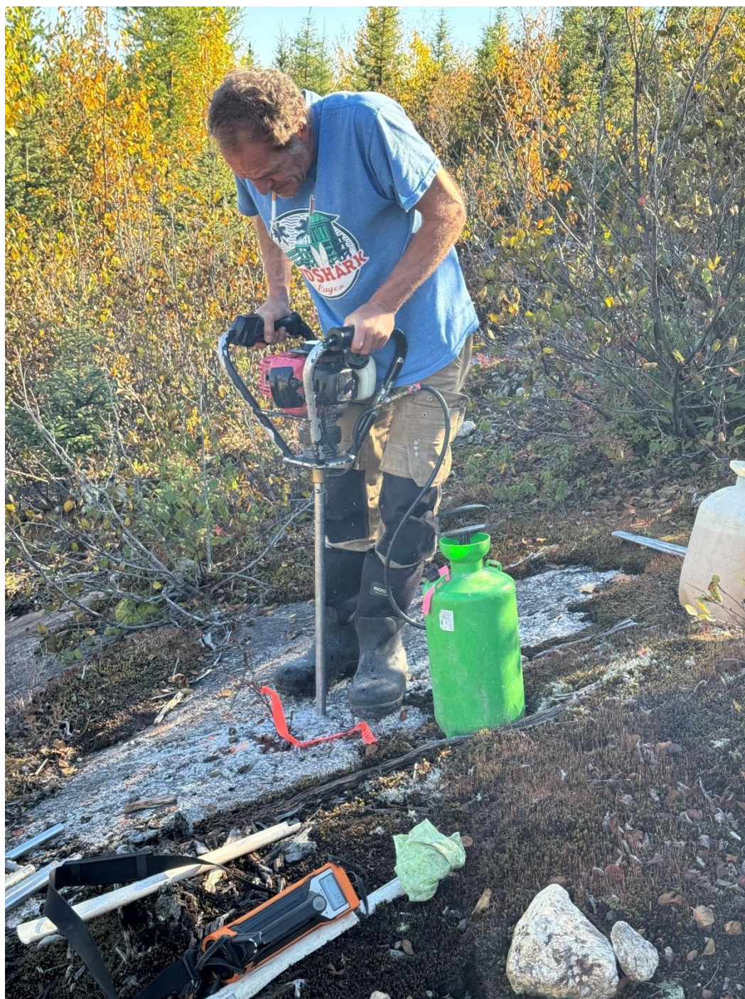
28.1.2 Drilling of duplicate “backpack drill” sample
