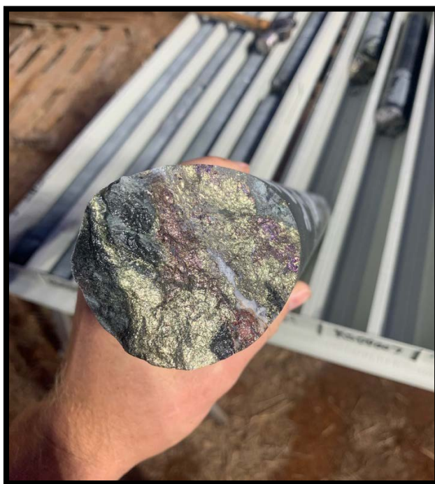
KSDD007 - 2cm thick bornite-chalcopyrite-quartz vein at 385m
