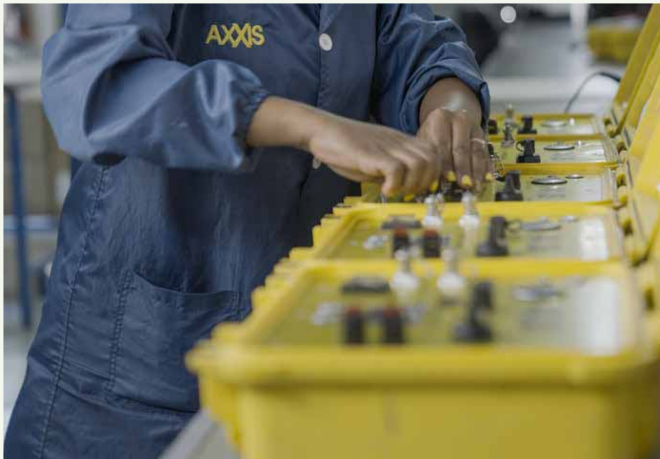
AXXIS Titanium™ allows up to 1 000 detonators to be initiated by each blasting box – reducing the amount of equipment that is needed on site
