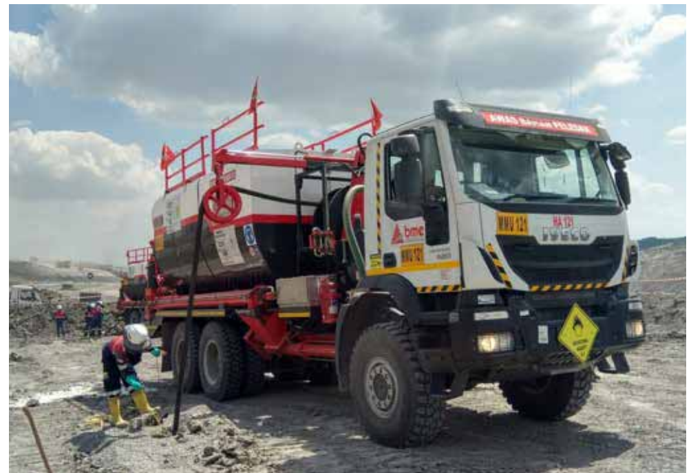
A BME Mobile Manufacturing Unit in Indonesia charging a hole, supporting our localisation approach to ensure supply security in core global markets.
