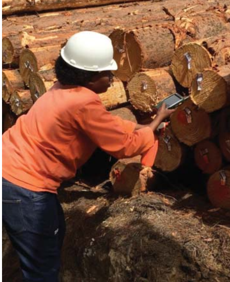
LogTrace scanner captures the details of the harvested product and the log is marked once it is scanned
