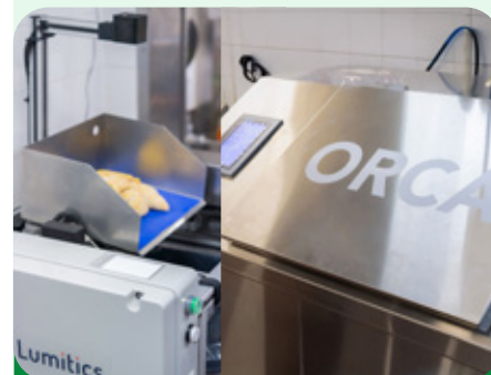
The Lumitics system and ORCA food waste digester analyze food waste patterns through AI technology
