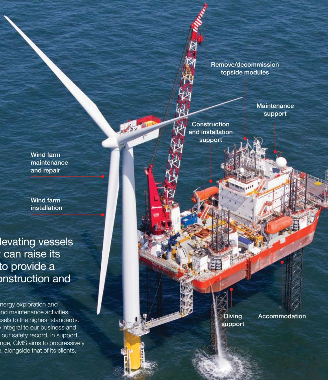
Self-propelled, self-elevating vessels are a mobile unit that can raise its hull above the water to provide a stable platform for construction and maintenance work.
