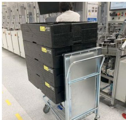
Adjustable-height lifting equipment deployed in Joyson Preh's Portugal Plant
