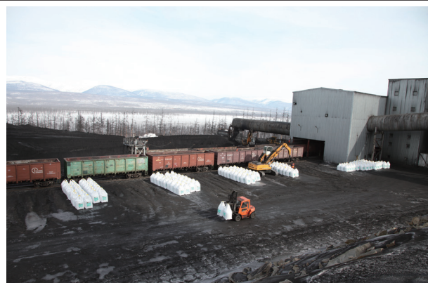
Loading of ilmenite product to wagons at Olekma
