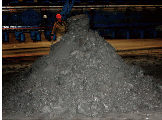
Wet iron ore concentrate after going through all stages of processing.
