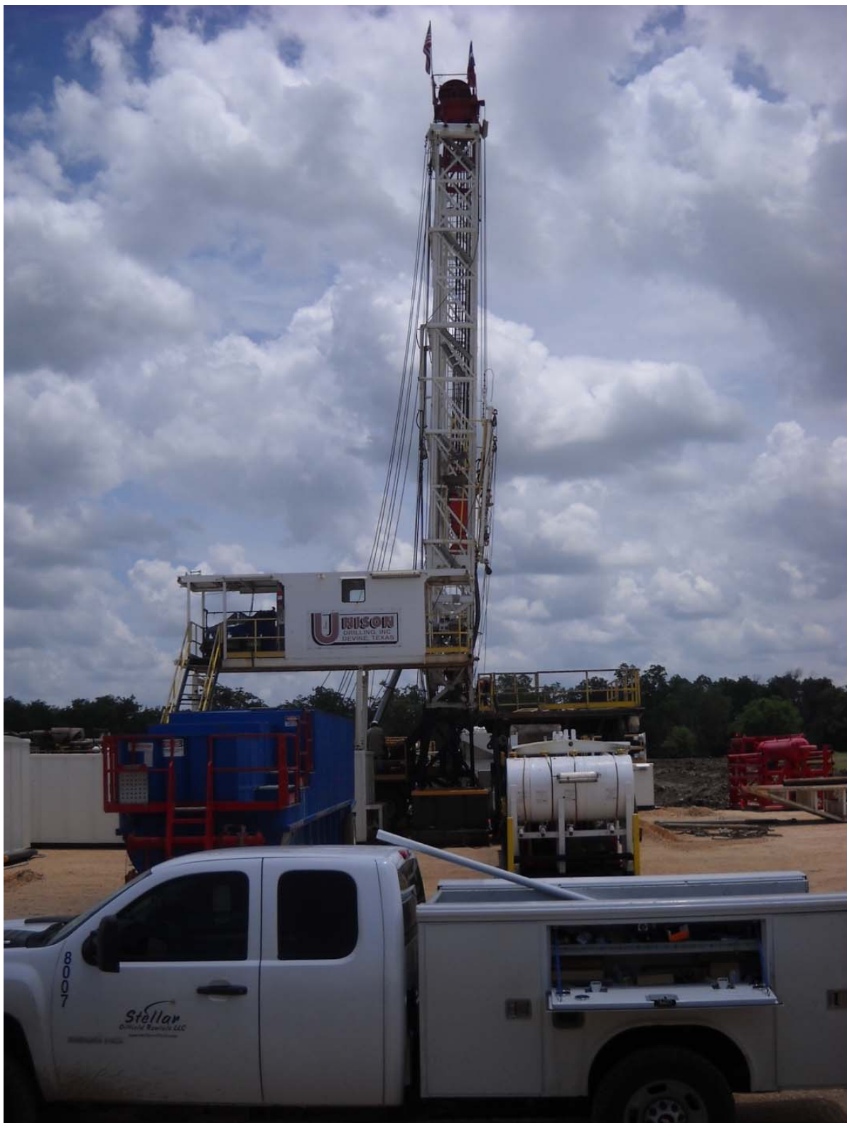
Photo 1 : Raising the oil drilling derrick prepping for rigging up the Nobel COG #1-H oil well on location Gonzales, Texas, June 2017.
