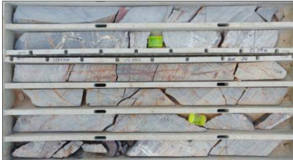
Figure 10-3 Example of core recovered from SHAK0007, also showing a zone of quartz-hematite veining
