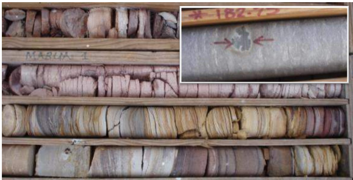
Figure 7-18 Dwyka tillite with sulphide accumulation in flaser-bedded siltstone (inset) in Mabua-2
