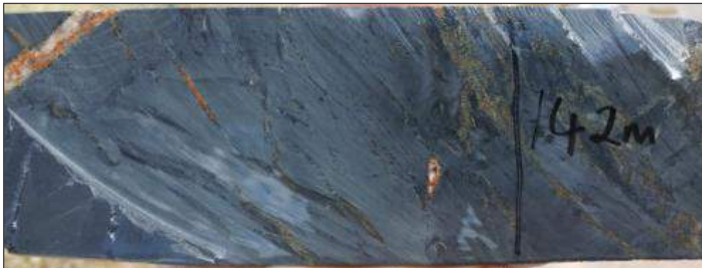
Figure 12-3 Veinlet-related pyrite-chalcopyrite mineralisation at 142 m in SHAK0007
