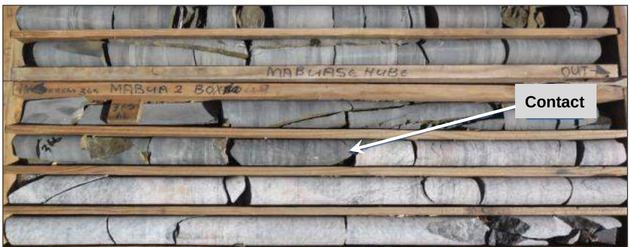
Figure 7-17 Faulted contact between pre-Karoo dolerite and underlying granitic gneiss basement in Mabua-2
