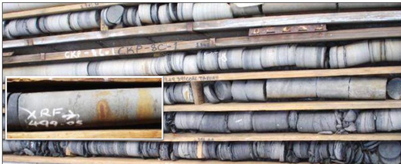
Figure 7-13 Ecce Group siltstone, minor arkose and carbonaceous shale and sulphide lenses (inset) in CKP-8C-1
