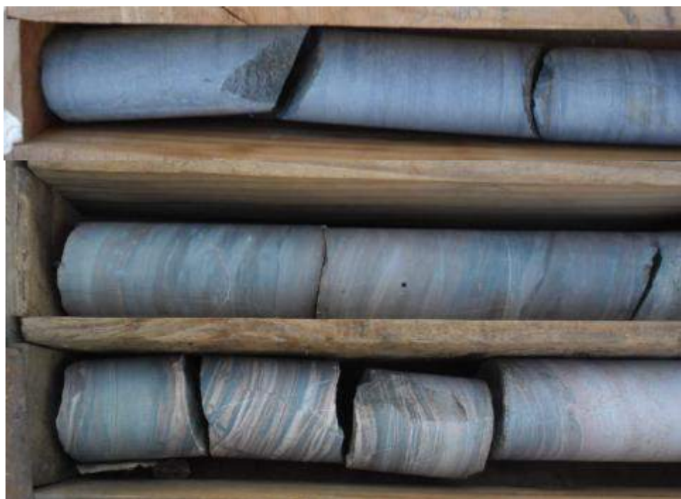
Figure 7-19 Gabbro with chilled margin (top row) and Transvaal chert with minor BIF (third row) in CKP-5C
