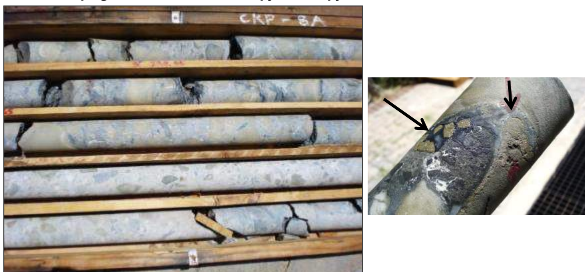
Figure 7-14 Slumping features and subhedral pyrite and pyrite rims (arrows in inset) in CKP-8A
