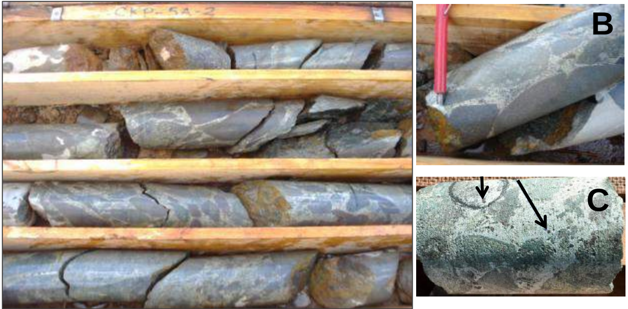
Figure 7-12 Volcanic breccia (agglomerate) with orientated clasts (B) and specks of native Cu (C) in CKP-5A-2
