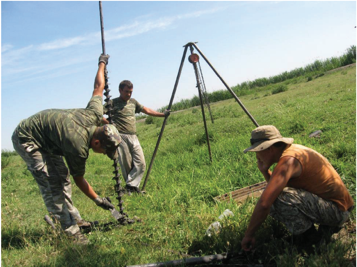
Figure 5-5: Manual Auger Drilling
