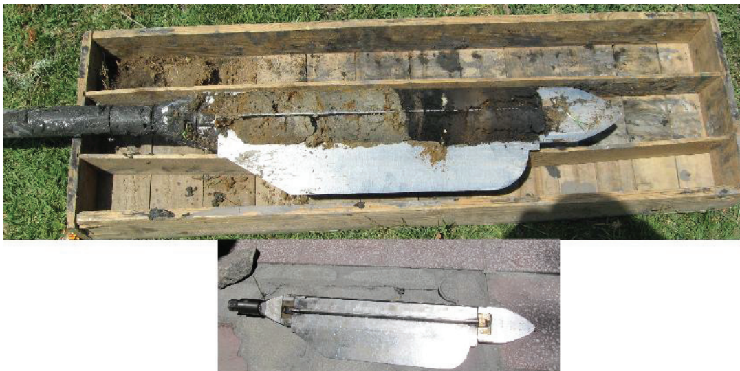
Figure 5-6: Sampling End of Manual Auger Designed to Ensure Maximum Sample Recovery and Minimise Contamination
