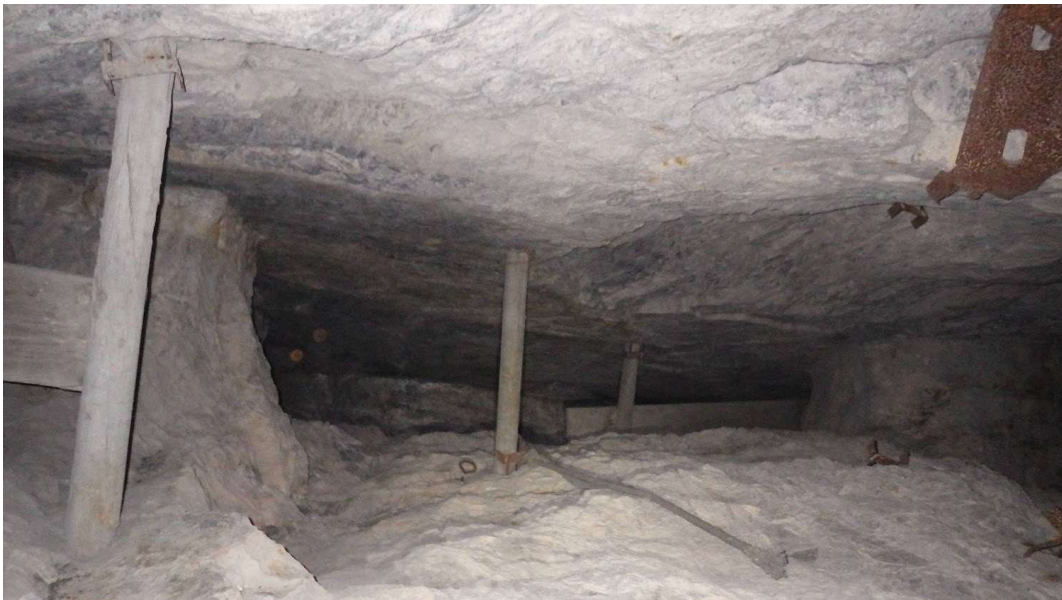
Figure 12-1: Image of old stope in Gold Prince mine, looking vertically up from Level 6, open and in reasonable condition
