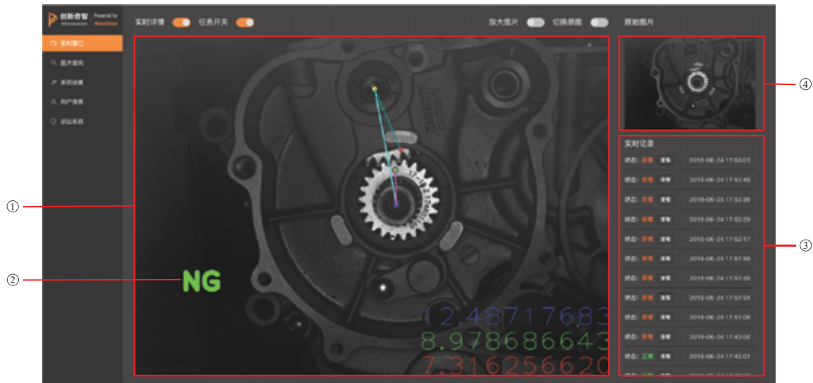
Defect detected in the production line as timing point not aligned
