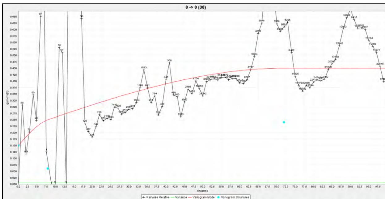
Figure 8-38 Northern Zone 100 Cu Along Strike (00°/000°) Pairwise Relative Variogram
