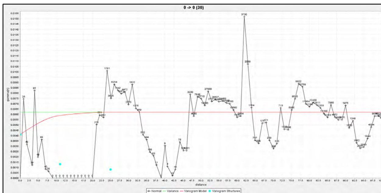
Figure 8-31 Northern Zone 102 Sn Along Strike ( 00^{\circ}/090^{\circ} ) Variogram
