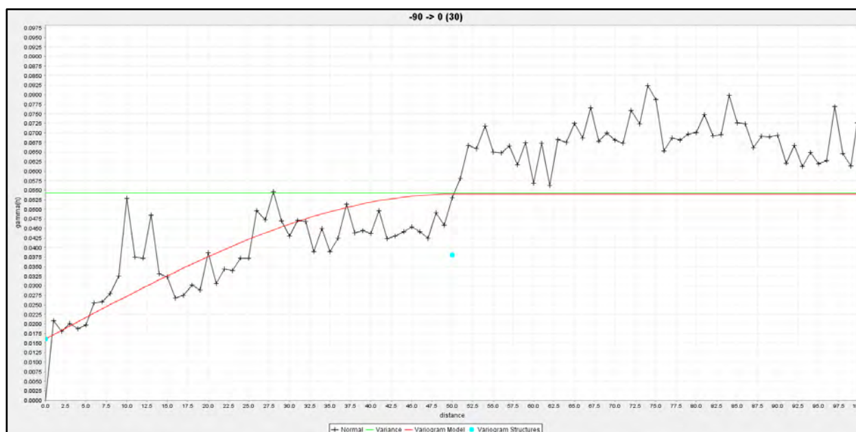
Figure 8-33 Southern Zone 200 Sn Down Dip (-90°/090°) Pairwise Relative Variogram
