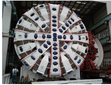
TBM Cutting Head ( Note )
