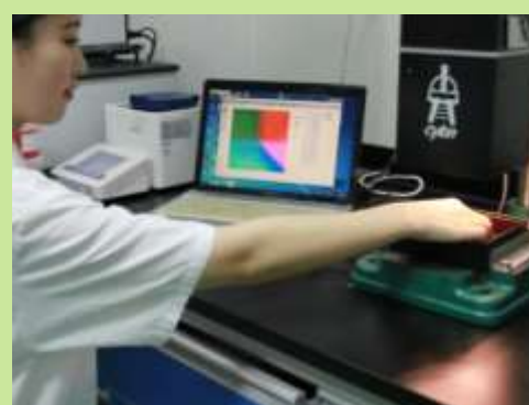
(3) Color difference meter – measured product's color
