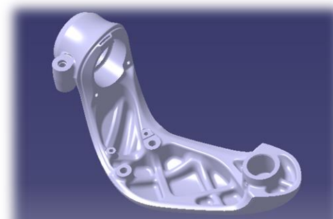
After Forging 1.782kg 6061 T6 Material Tensile Strength 310Mpa
