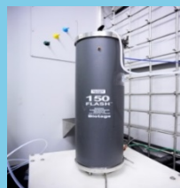
6 inch MPLC system
