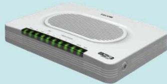
GPON IAD with RF Overlay
