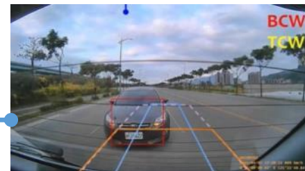
Rear Side road rage detection 後方危險駕駛偵測提醒
