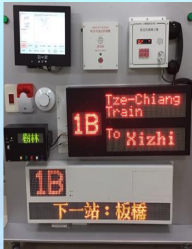
Carriage Automatic Broadcasting System
