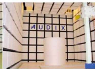
RF全電波暗室 RF ETSI Fully Chamber
