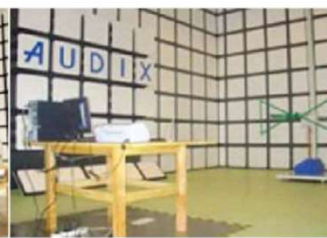
輻射干擾測試實驗室 (3米法半電波暗室) 3m Semi-Anechoic Chamber
