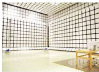
輻射干擾測試實驗室 (10米法半電波暗室) 10m Semi-Anechoic Chamber
