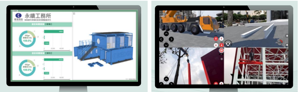
BIM combined with the application of GHG inventory and BIM steel engineering simulation hoisting
