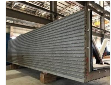
Precast exterior wall (rubber mold concrete)
