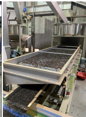
-> Drying -> Grinding -> 4 stage fine screening -> Winnowing 、 Color Sorting -> Blending -> Q.C -> Storage
