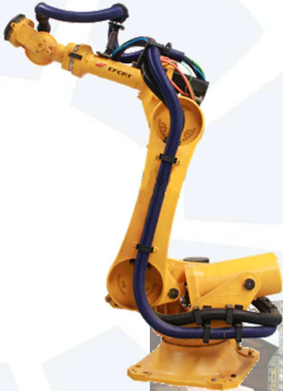
Cable for connection between control cabinet & robot arm
