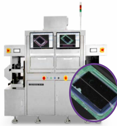
TR7900Q SII-R Magazine & Strip + Reject Station 3D Semi AOI
