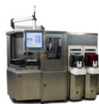
eWLB wafer de-bonding Warpage Adjustment
